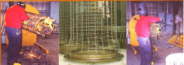
HawkeyePedershaab's Model QRE Cage Machine is an economical machine that brings the efficiency of machine-manufactured reinforcement within the reach of virtually any producer.
