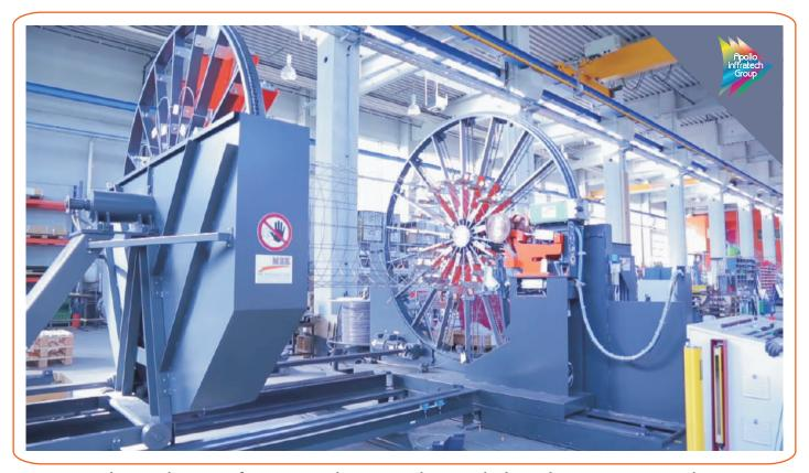
For the production of wire cages being used in manhole and concrete pipe industry [Product range from 330mm to 2500mm diameter and up to 3000mm length]
